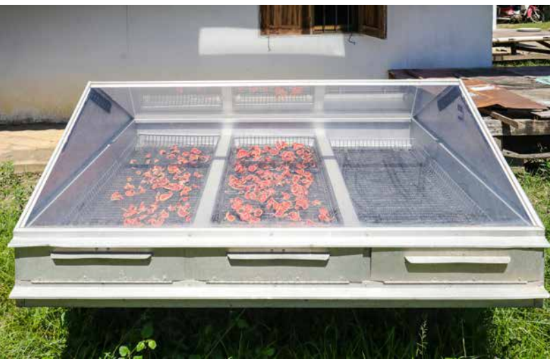
Figure 1. Example of a solar dryer used to preserve fish and meats.
