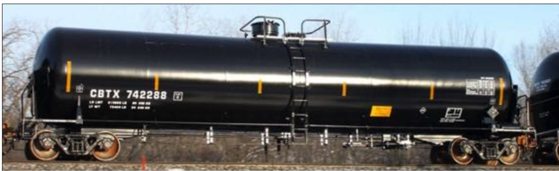
Figure 7: DOT-111 Tank Car
