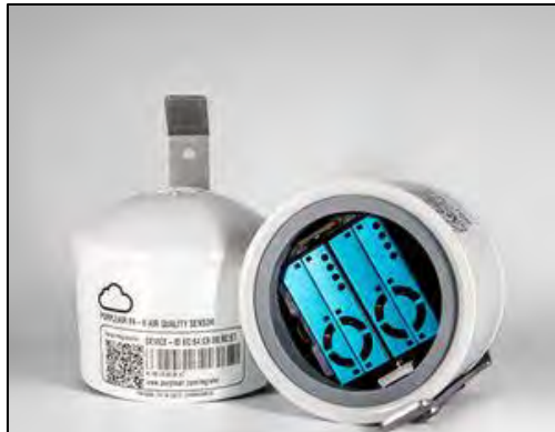
Dual internal sensors allow for error checking
